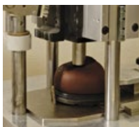
Above: The weight is dropped onto the protective toe cap area.
