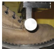
Above: The weight is dropped on the protected metatarsal area.
