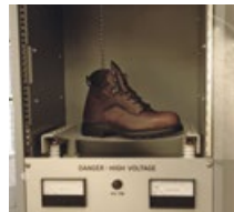
Above: The boot is placed on the metal mesh platform. The gauges measure leakage through the footwear.
