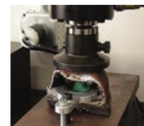
Above: The toe cap is being compressed between the parallel platens.
