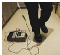
Above: The tester steps on the base electrode plate while the electrical resistance is measured.
